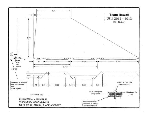
Both the fin, and its associated fin-can, are made using annealed 6061 Aluminum (0.4-0.8% Si, <0.7% Fe, 0.15-0.40% Cu, < 0.15% Mn, 0.8-1.2% Mg, 0.04-0.35% Cr, <0.25% Zn, <0.15% Ti), having a density of 2.70 grams per cubic centimeter, a Young's modulus of 10 Mega-psi, a maximum tensile strength of 18,000 psi, a maximum yield strength of 8,000 psi, and an elongation (stretch before ultimate failure) of 25-30%.
