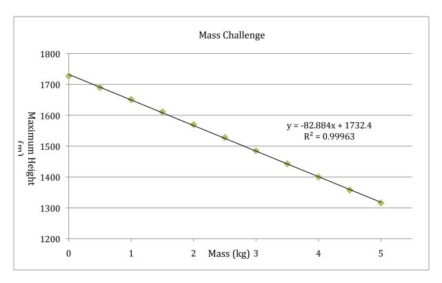
What is clear is that, if possible, the mass of the payload (and any other incidental mass increase) should be less than 1.5 kg in order for us to reach one mile altitude (1625 m).
