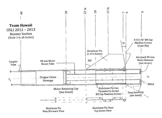
An Aeropack 98-mm motor retainer will be attached to the aft bulkhead by means of 6 nut and bolt assemblies. What is not clearly shown is the Motor Retaining Cap (MRC). It is at the MRC where the final U-bolt is placed. This is where the shock cord joining the avionics section, and associated with the main chute, is attached.
