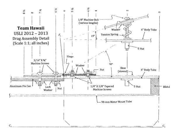
One observation that should be mentioned is that when the drag shoes are deployed, the CP of the rocket is lowered (~3% at full deployment, using center of area estimates), and enhances the stability of the rocket. Subsequent testing of our expectations, using a 1:3.7 scale model has been done, and has confirmed a loss of ~1% of altitude for every degree that the drag shoes are deployed.
