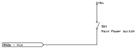
Note #1: The main power switch is located on 4 AAA Battery Holder (Radio Shack part # 270-411)
