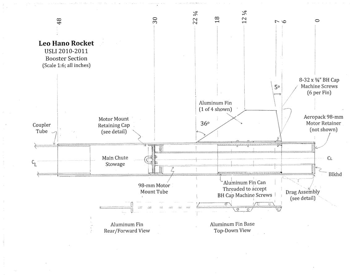
The major change to the booster construction was the removal of the fore centering ring, and replacing it with a Motor Mount Retention Cap. Of concern to the team
